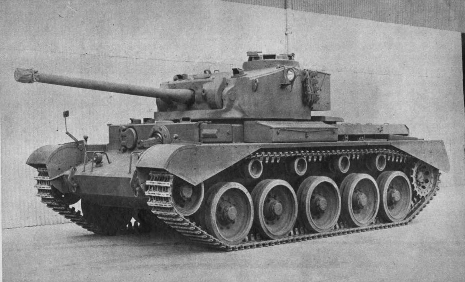
NEW COMET HAS CAST TURRET FRONT WITH BULGING GUN MANTLET, PROMINENT CUPOLA. NOTE THE FIVE BOGIES, FOUR RETURN ROLLERS
